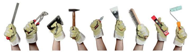
Hammers, wrenches, chisels, pliers, screwdrivers, and other hand tools are often underrated as sources of potential danger. Hand tools may look harmless, but they are the cause of many injuries. In fact, an estimated 8 percent of all workplace compensable injuries are caused by incidents associated with hand tools. These injuries can be serious, including loss of fingers or eyesight.
